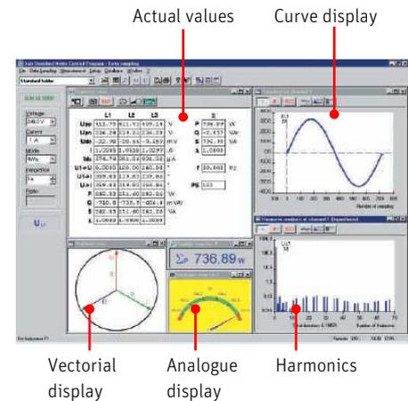
All relevant data (parameters and control codes for the item under test, switch-on sequence, tolerance ranges etc.) are stored in databases. The test results from databases can be statistically analyzed with the SSM3000 software protocol function, printed out in the different display forms, and exported into MS Excel files.
